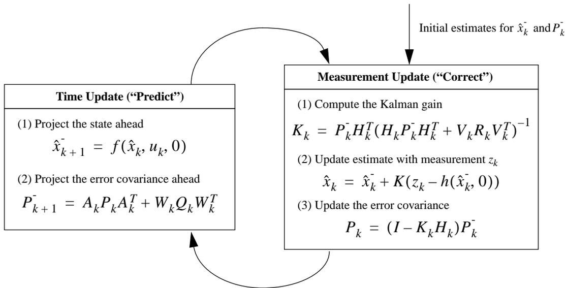
**Figure 2-1.** A complete picture of the operation of the *extended* Kalman filter, combining the high-level diagram of Figure 1-1 with the equations from Table 2-1 and Table 2-2.
