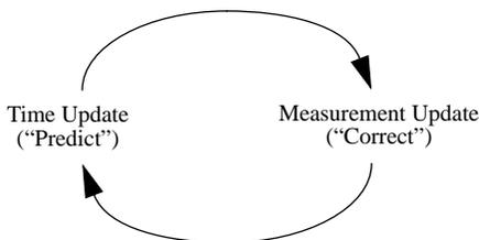
**Figure 1-1.** The ongoing discrete Kalman filter cycle. The *time update* projects the current state estimate ahead in time. The *measurement update* adjusts the projected estimate by an actual measurement at that time.
