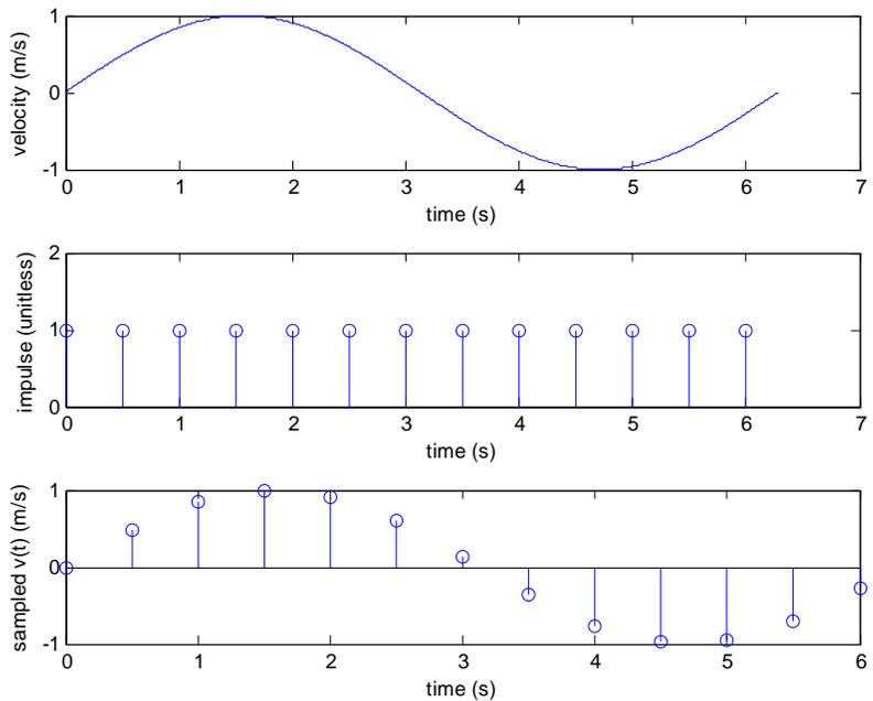
Performing this operation is known as "sampling" the function  $v(t)$  at the sampling frequency of  $1/\Delta T$ , where  $T$  is the period of the impulse train. Note that an impulse train can also be written as
