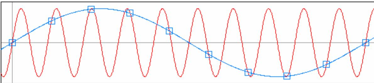
“Two different sinusoids that give the same samples; a high frequency  $f > f_s/2$  (red) and an alias at  $f_s - f$  (blue).” (<http://en.wikipedia.org/wiki/Aliasing>, accessed 10/05/06).
