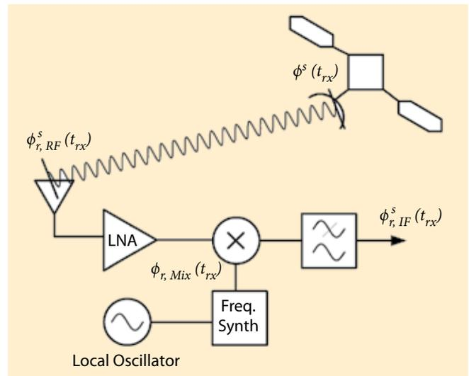
**FIGURE 1** Signal phase from transmission through downconversion to intermediate frequency. At each point the signal is assumed to be a sinusoid, the phase of which is indicated in text in the figure.
