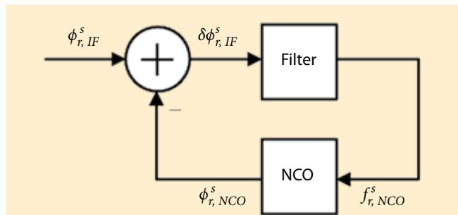
FIGURE 2 Linear model of a phase locked loop (PLL). A local replica sinusoid with phase  $\phi_{r,NCO}^s$  is generated by a numerically controlled oscillator (NCO). The difference between this local replica and the IF phase is filtered to generate a command signal for the NCO  $f_{r,NCO}^s$ , which drives the error signal  $\delta\phi_{r,IF}^s$  to zero.
