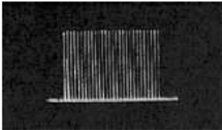
**Fig 5: Spectrum of a FHSS Signal**
