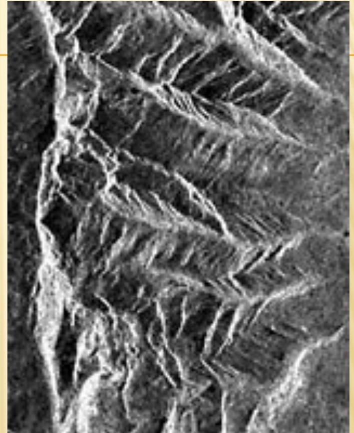
Layover occurs when the radar beam reaches the top of a tall feature before it reaches the base. The top of the feature is displaced towards the radar sensor and is displaced from its true ground position - it 'lays over' the base.
