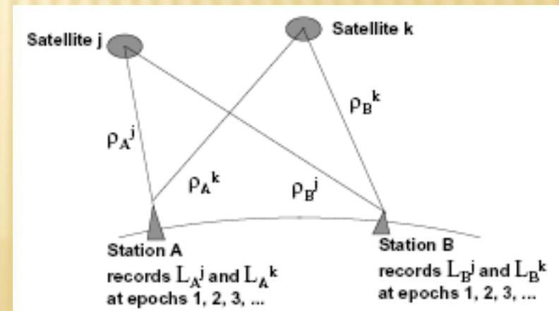
$$\nabla \Delta L_{AB}^{jk} = \Delta \rho_{AB}^j - \Delta \rho_{AB}^k + \Delta c \tau_{AB} - \Delta c \tau_{AB} \\ + \Delta Z_{AB}^j - \Delta Z_{AB}^k + \Delta I_{AB}^j - \Delta I_{AB}^k + \Delta B_{AB}^j - \Delta B_{AB}^k$$
