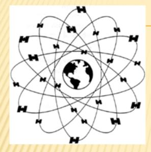
24 satellites in 6 orbital planes. Carry highly stable atomic clocks to generate GPS signals (GPS really measures time, not distance)
