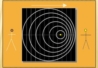
See higher frequency when XTR moving towards The change in the rate of phase change (fixed change in frequency) observed at receiver, with respect to stationary transmitter, is proportional to velocity of moving transmitter.
