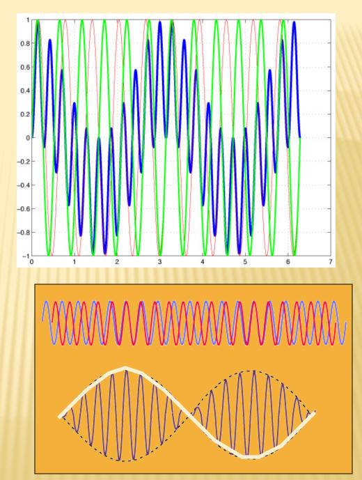
In terms of our GPS signals we get (we are now mixing – multiplying, not adding. G= GPS signal, R= Reference signal.)
