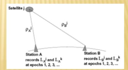
$$\begin{split} \Delta L_{AB}^{j} &= L_{A}^{j} \left( T_{A} \right) - L_{B}^{j} \left( T_{B} \right) \\ \Delta L_{AB}^{j} &= \rho_{A}^{j} - \rho_{B}^{j} + c\tau_{A} - c\tau_{B} - c\tau^{j} + c\tau^{j} \\ &+ Z_{A}^{j} - Z_{B}^{j} - I_{A}^{j} + I_{B}^{j} + B_{A}^{j} - B_{B}^{j} \end{split}$$
