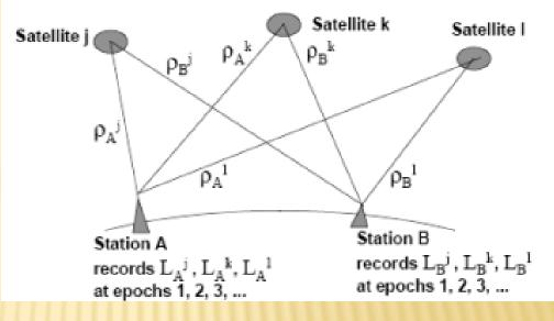
Note that we can form any one from a linear combination of the other two  $L_{AB}^{jk} = L_{AB}^{jl} - L_{AB}^{lk}$  $L_{AB}^{jl} = L_{AB}^{jk} - L_{AB}^{lk}$  $L_{AB}^{lk} = L_{AB}^{jk} - L_{AB}^{jl}$
