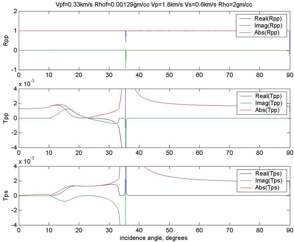
Figure 2: Real and imaginary parts of RPP, TPP, and TPS as a function of incidence angle in the incident pressure.
