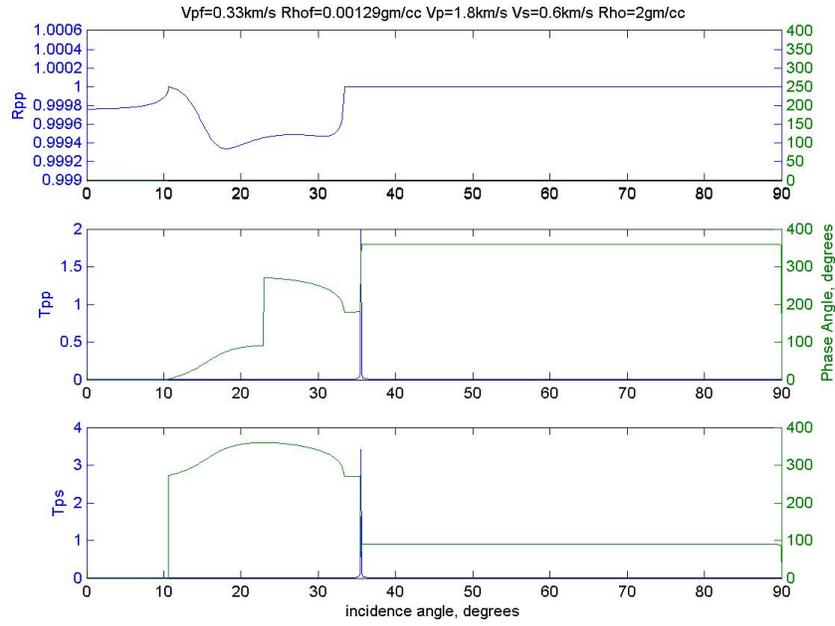
Figure 3: Amplitude and phase of the three reflection and transmission coefficients plotted at full scale.
