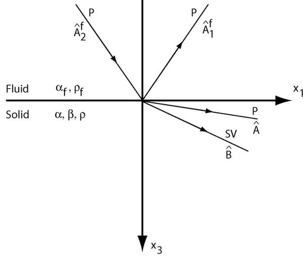
Figure 1: Incident P wave from upper left interacting with a fluid/solid boundary.
