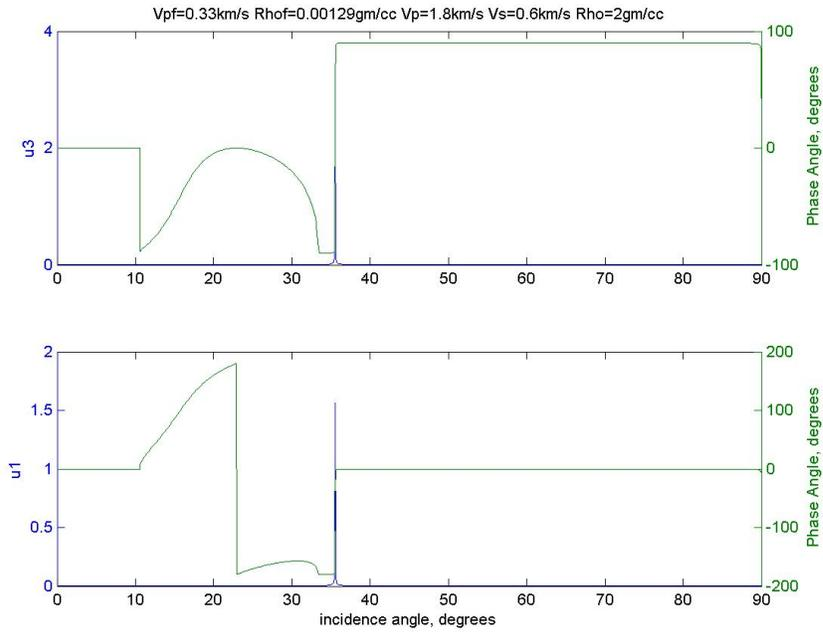
Figure 7: Amplitude and phase at full scale for the vertical and radial displacements in the solid medium.
