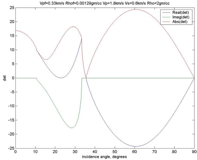
Figure 4: Behavior of  $\det D$  (equation 15) with incidence angle. There is a minimum (but not a zero) near  $35.5^\circ$ .
