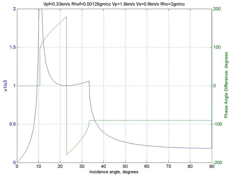
Figure 8: Ratio of the radial to vertical displacement amplitude at the interface. Also shown is the phase difference between the radial and vertical displacements.
