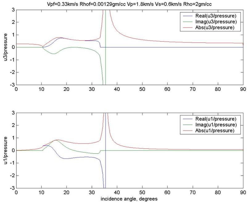
Figure 9: Ratio of the surface displacements to the total pressure field in the fluid. Units are in microns/Pa. The maximum of the ratios at the Stonely wave pseudo-pole are 1243 and 722 for  $u_3/\text{pressure}$  and  $u_1/\text{pressure}$ , respectively. The factor of  $1/i\omega$  has not been included in these plots and it should be understood that the displacement time histories are the time integral of the incident pressure time history.
