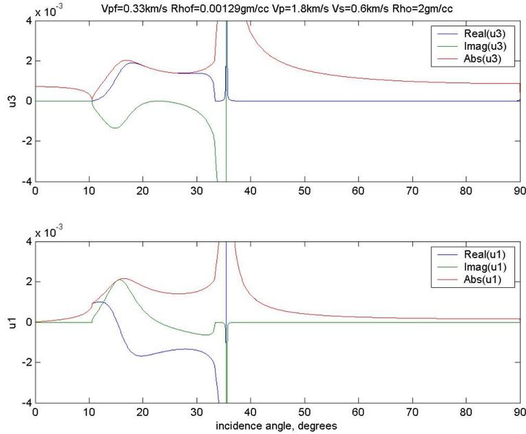
Figure 6: Real and imaginary parts of the vertical and radial displacements in the solid medium.
