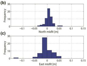
*filled circles*. **b** Histogram of north component differences shown in **a**. **c** Histogram of east component differences shown in **a**
