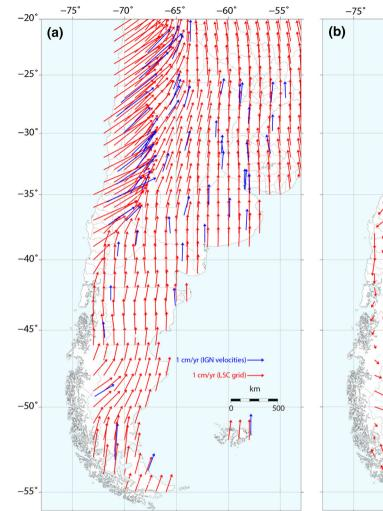
**Fig. 2** a Least squares collocation of the secular inter-seismic velocities of the RAMSAC, CAP and IGS networks in POSGAR07. *Blue arrows* show the CGPS stations used for the interpolation. *Red arrows* show the 1° grid in latitude and longitude of interpolated velocities. **b**
