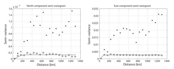
Fig. 3 Semi-variogram plots of the north and east components of the post-seismic transient after applying an exponential taper detrending function. *Empty circles* show the detrended data, *filled circles* show the original data, and the *solid line* is the Gaussian semi-variance model
