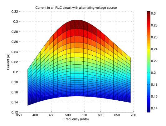
Figure 43: Current in an RLC circuit with alternating voltage source
