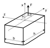
Figure 22: Cross section of a rectangular beam
