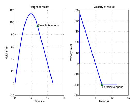
Figure 48: Speed and altitude of a rocket
