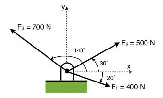
Figure 15: Forces on a bracket
