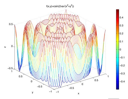
Figure 11: Surface plot (using mesh) of the function  $z = c \cdot \sin(2\pi a \sqrt{x^2 + y^2})$
