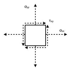
Figure 27: A 2D state of stress at a point in a loaded material
