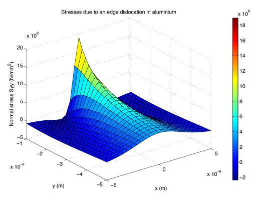
Figure 39: Normal stress  $\sigma_{yy}$  due to an edge dislocation in a luminium
