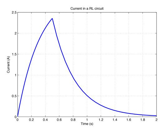
Figure 31: Current in a RL circuit
