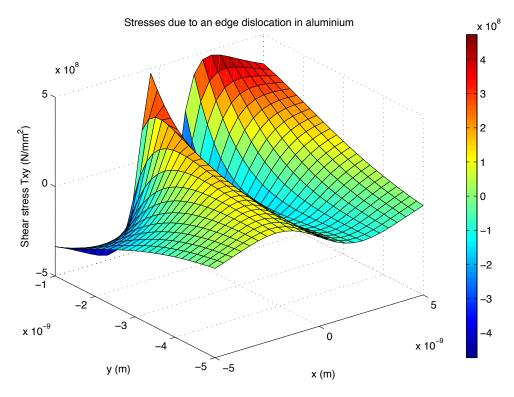
Figure 40: Shear stress  $\tau_{xy}$  due to an edge dislocation in a luminium
