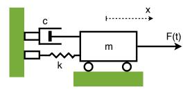
Figure 20: Modelling helicopter rotor vibrations with spring-mass-damper system
