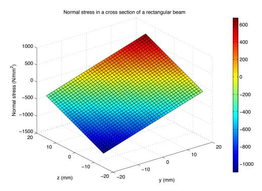
Figure 37: Normal stress in a cross section of a rectangular beam
