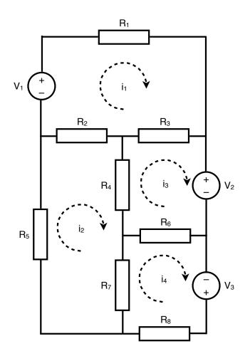
Figure 17: Network of voltage sources and resistors
