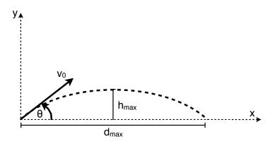
Figure 26: Motion of a projectile
