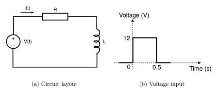
Figure 19: RL circuit
