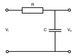
Figure 28: A low-pass filter
