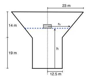
Figure 14: Water level in a water tower
