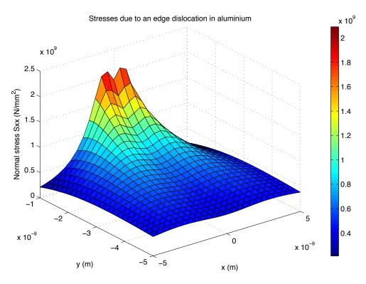
Figure 38: Normal stress  $\sigma_{yy}$  due to an edge dislocation in aluminium
