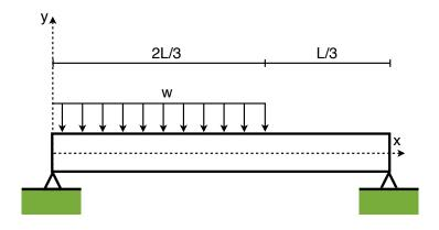
Figure 21: A simply supported beam
