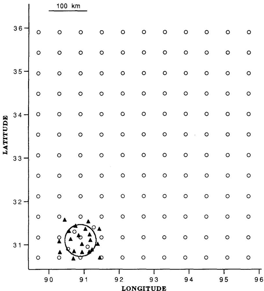
FIG. 2. Distribution of stations (solid triangles) and epicenters (open circles) for Tests 1, 2, and 3. For Test 4 only the stations inside the circle were used.
