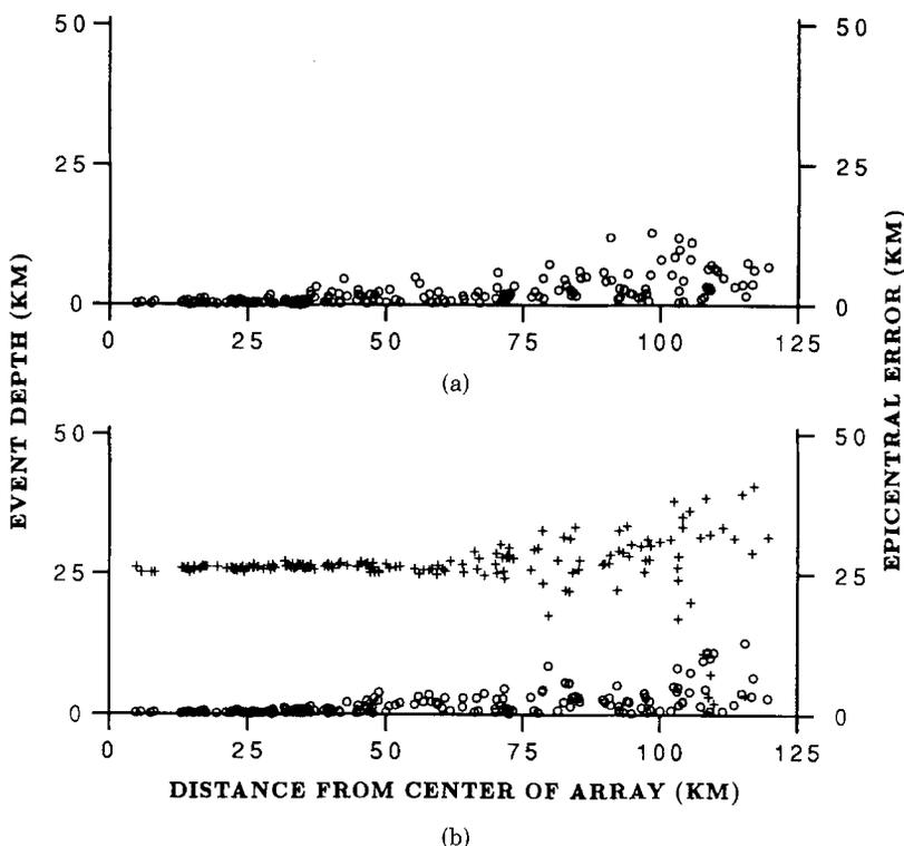
FIG. 6. Summary of results of Test 4. Depth of the events 25 km. Errors added to the arrival times. Symbols as in Figure 3. (a) Errors in the epicenters computed by the epicentral location routine. (b) Depths and errors in the epicenters computed by the hypocentral location routine using both *P* and *S* arrivals.
