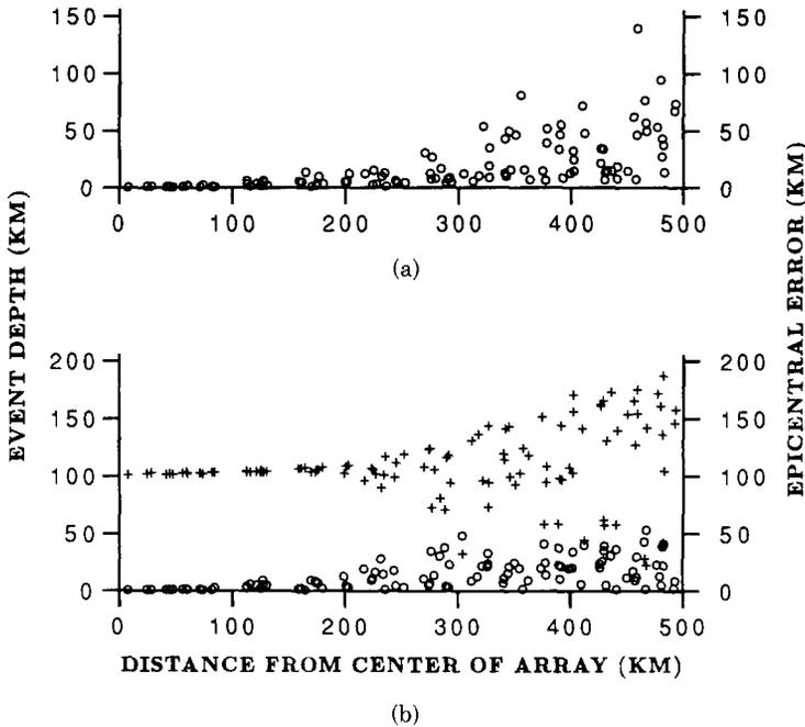
FIG. 4. Summary of results of Test 2. Depth of the events is 100 km. Errors added to the arrival times. Symbols as in Figure 3. (a) Errors in the epicenters computed by the epicentral location routine. (b) Depths and errors in the epicenters computed by the hypocentral location routine using both *P* and *S* arrivals.
