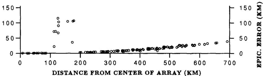
FIG. 5. Results of Test 3. Errors in the epicenters computed by the epicentral location routine. Depth of the events 25 km. Error-free data. Symbols as in Figure 3. The large epicentral errors between 100 and 200 km are caused by the mixing of direct and head wave arrivals.
