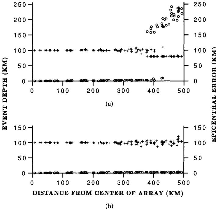
FIG. 7. Depths and errors in the epicenters for the events of Test 2 located with HYPOINVERSE. Both *P* and *S* arrivals were used. Symbols as in Figure 3. (a) An initial depth of 80 km was given. For events beyond about 380 km, depths remain unchanged, an indication that the program failed to converge. (b) The approximate locations and origin times were used as initial solutions.
