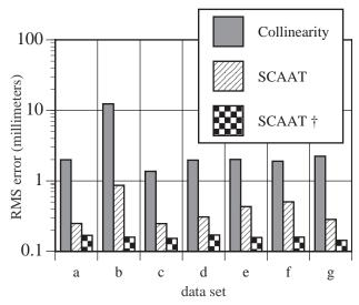
Figure 7: RMS error results for simulations of all seven real user motion data sets. The † symbol indicates a second pass through the motion data set, this time using the already autocalibrated beacons.
