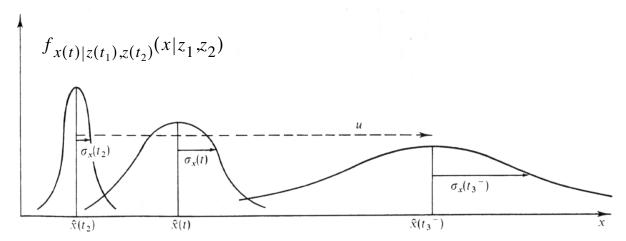
FIG. 1. 7 Propagation of conditional probability density.
