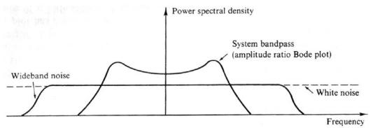
FIG. 1. 3 Power spectral density bandwidths.
