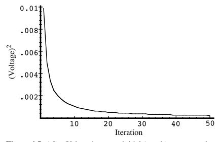
**Figure 4.5:** After 50 iterations, our initial (rough) error covariance  $P_k$  choice of 1 has settled to about 0.0002 (Volts<sup>2</sup>).
