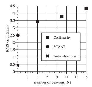
Figure 5: As the number of beacons N is reduced from 15 to 5, the Collinearity results improve slightly. (The Collinearity algorithm generally becomes unstable with  $N \le 4$ .) The SCAAT results, with N=1 beacons, are better, and especially good once autocalibration is turned on.
