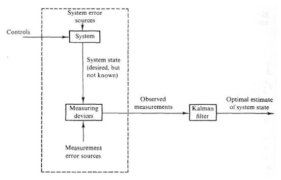
FIG. 1. 1 Typical Kalman filter application
