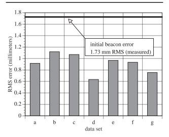
Figure 8: Autocalibration in action. Here we show the final beacon position error for runs through each of the seven user motion data sets.
