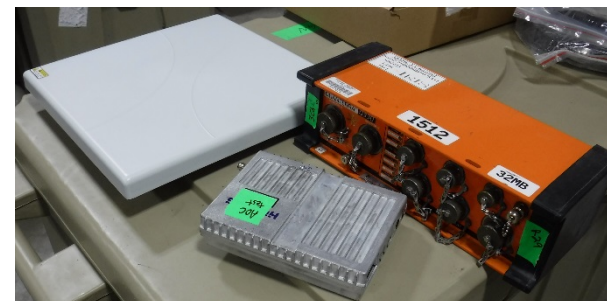
BGAN terminal and panel antenna with Q330 for scale
