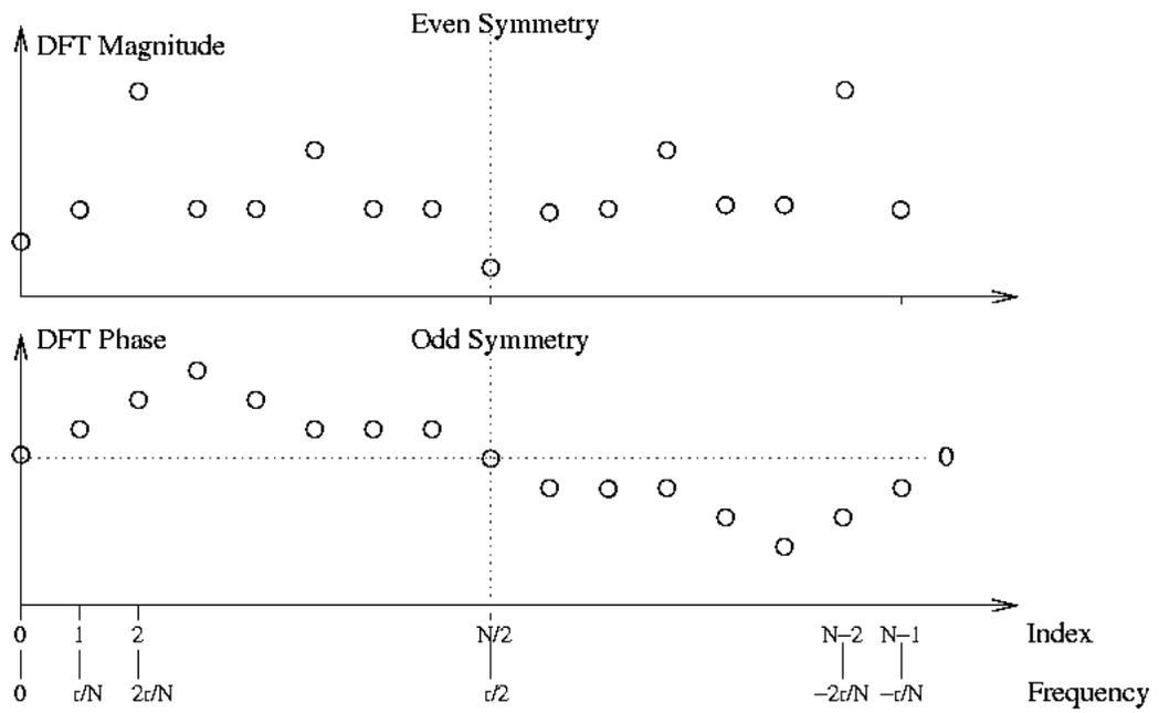
Figure 4: DFT frequency-index mapping.
