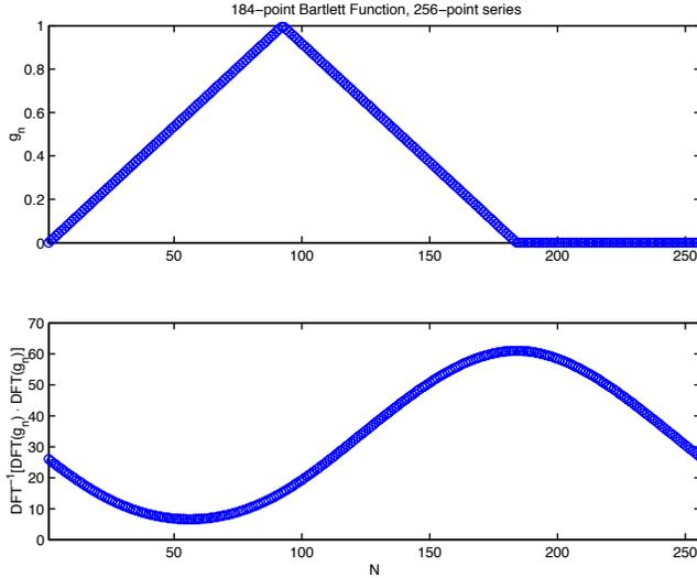
Figure 5: Wraparound in an  $N = 256$ -point Circular Convolution.
