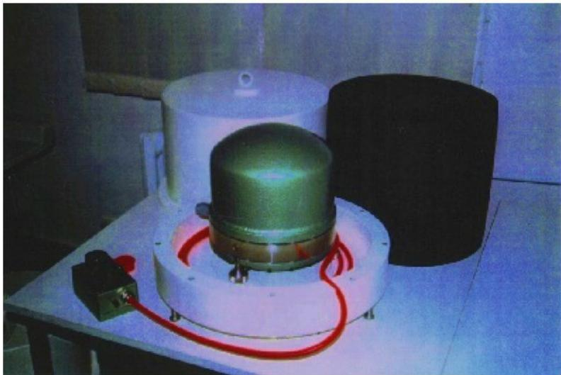
Figure 13: An STS2 seismometer.
